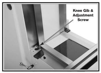
Figure 60. Knee gib and adjustment screw.
